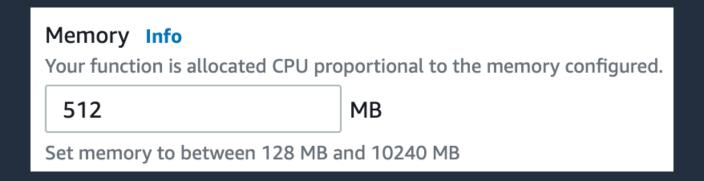
CPU capacity is allocated proportionally to the amount of allocated memory
