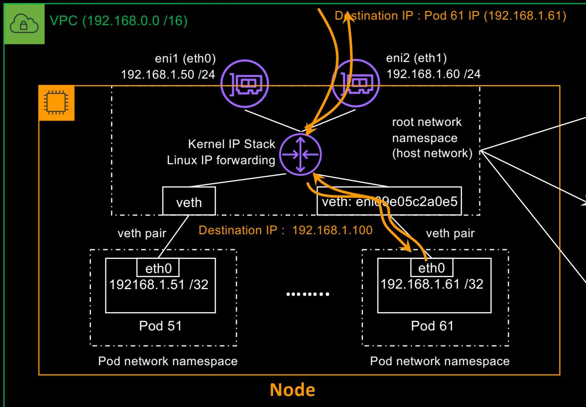
eni specific route table (to route Pod's outgoing traffic) (since each pod is using an IP from the respective eni)
