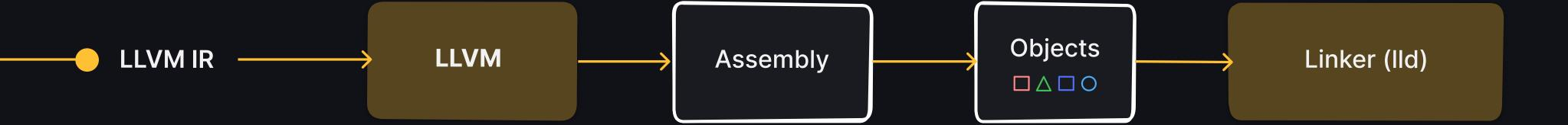
**Code Generation** involves generating the machine code for the specific platform by LLVM. **LLVM IR** is assembly-like with additional low-level types and annotations added for optimizations.
