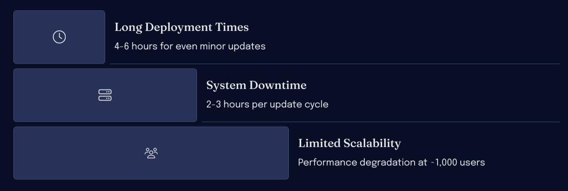
Traditional monolithic architectures require complete redeployment for even minor updates, leading to significant operational inefficiencies. These systems are particularly vulnerable to scalability issues as all components are interconnected and interdependent.
