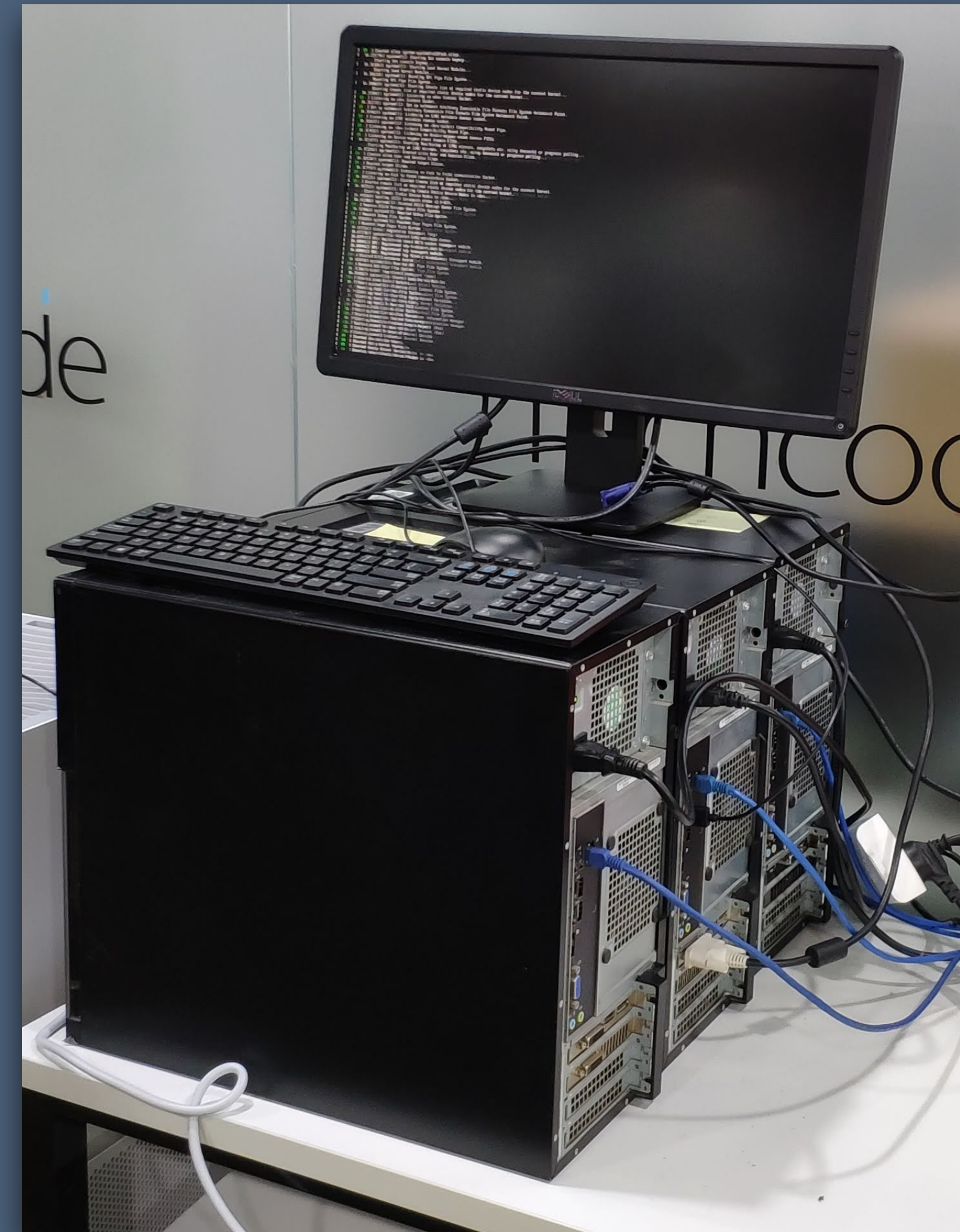
An affordable ML Platform running on 3 PCs with 3 RTX1060
